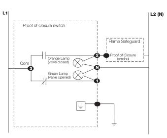
Do not wire the valve switch to close a circuit that will directly power another safety shutoff valve. Doing so could result in a safety valve being energized and opened rather than remaining closed.
